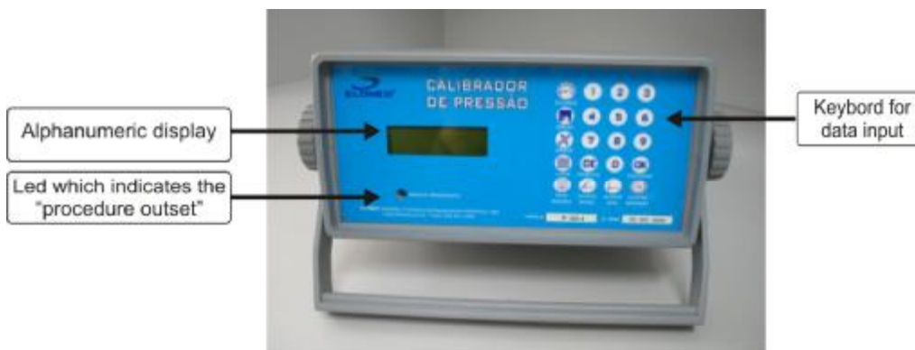
Figure 1 Pressure gauge with details of the alphanumeric display, keyboard for data input and led functioning signalizer
