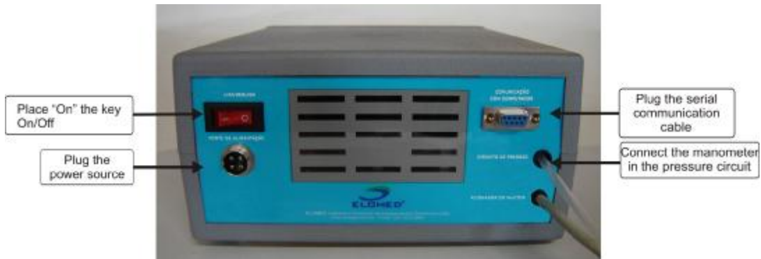
Figure 3 View of the back side of the pressure gauge and description of the parts
