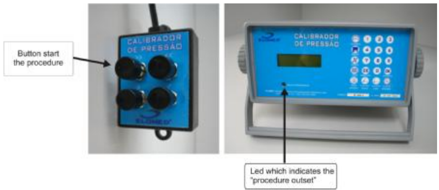
Figure 9 Detail of the button to be powered to start the gauging and signalization led of the "procedure outset"
