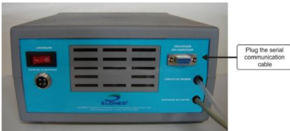
Figure 16 Connection with the computer through the serial port.
